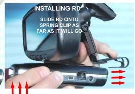
7 - When removing or installing the RD, squeeze the trigger and the back side of the mount together with one hand, and lift the front of the RD upward with the other hand before sliding the RD off or onto the spring clip. You must lift the front of the RD upward before sliding it off or onto the mount.
